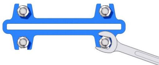
If the glandfollower nuts are overtorqued, the force needed to operate the valve will increase, the valve function will be affected and the box packing lifetime will be shortened.
